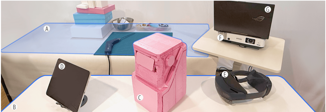
Figure 8: The constructed IEDS environment. ① physical prototype building area: providing physical prototype materials and common tools; ② prototype augmentation area: in which a blank table is provided for virtual editing and prototype discussion; ③ current version of the built physical prototype for discussion; ④ the tablet computer (for GAI+HHD); ⑤ the HMD equipment (for GAI+HMD); ⑥ the projector (for GAI+SAR); ⑦ the computer for connecting the projector, head mounted display equipment, and back-end server. Note: IEDS supports multi-person collaboration, with more than one tablet computer and head-mounted display equipment in the design space. Only one piece of equipment is shown as an example.
