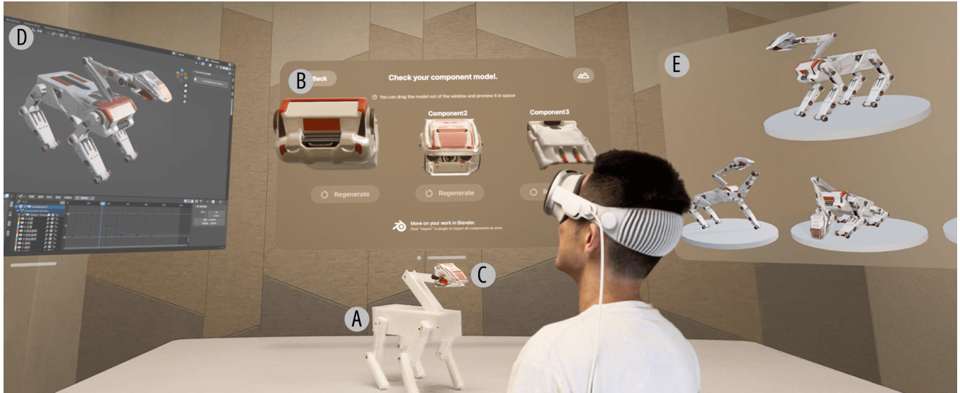
Figure 1: A prototype process supported by FusionProtor. ①: The designer constructed and interacted with a physical prototype embodied. ②: He utilized FusionProtor to generate component-level 3D prototypes based on the low-fidelity physical prototype. ③: He coupled the physical prototype with virtual components for mixed iteration. ④: He assembled 3D components and simulated their interaction according to physical motion logic. ⑤: FusionProtor's 3D design outcome and simulation presentation.
